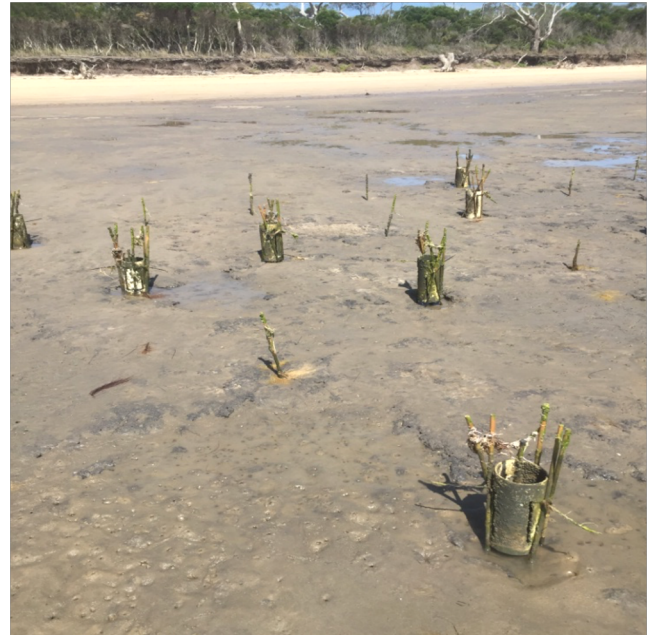
Figure 6. Erosion beneath and surrounding protective tubes on Plot X1.
