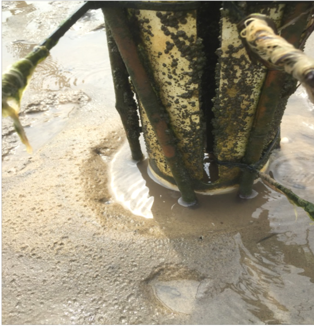
Figure 6. Erosion beneath and surrounding protective tubes on Plot X1.
